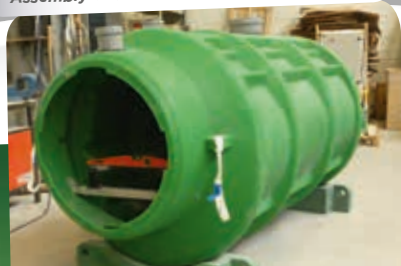
Assembly of the STAR1000 pumping stations
