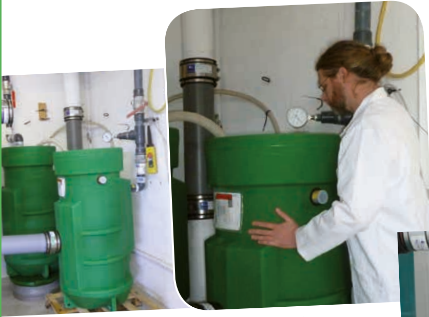
Tests bench: control of the specifications of a pumping station
