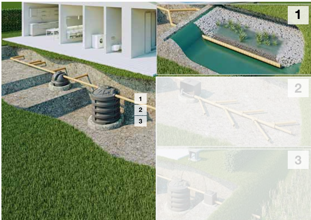
Figure 10 Plant for domestic use, drain into the ground composed of the DG, IMHOFF, 1) EVAPO models
