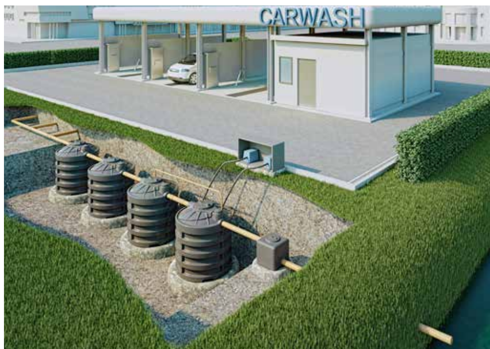
Figure 13 Complete car wash systems with drainage into surface water
