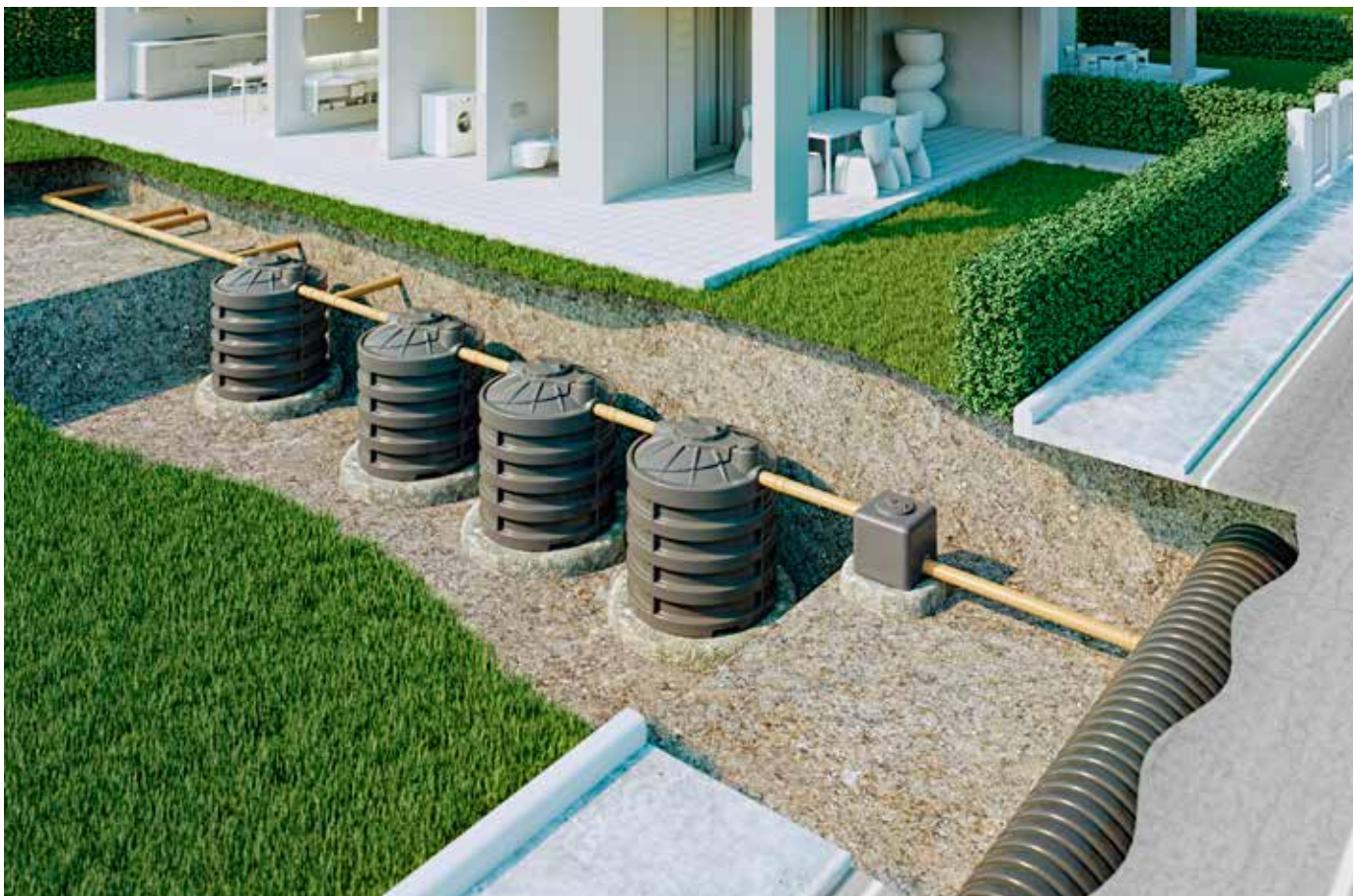
Figure 1 Installation in series of model ST for domestic use, drainage into public sewers
