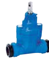
Series 03/90 Service connection valve with PRK couplings for PE pipes DN20-50 PN16 Ductile iron
