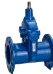
Series 02/75 Flanged gate valve Face-to-face DIN F5 Replaceable stem sealing DN40-500 PN10/16 Ductile iron
