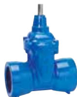
Series 33/00 Gate valve with socket ends for cast iron pipes DN80-300 PN16 Ductile iron With internal enamel
