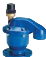
Series 701/50 Combination air valve Inlet flange DN50-300 PN16 Grey cast iron/ Reinforced polyamide
