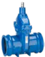
Series 01/80 Gate valve with "Euro" socket ends for uPVC-pipes DN40-400 PN16 Ductile iron
