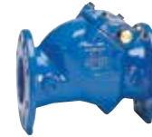
Series 41/61 Swing check valve Resilient seated Closed bushings DN50-300 PN10/16 Ductile iron
