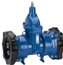
Series 636 Supa Maxi™ gate valve Universal and tensile coupling ends for all pipes DN80-300 PN16 Ductile iron
